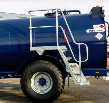
LARGE FLOTATION TYRES FOR OFF-ROAD USE GALVANISED REFUELLING PLATFORM (6000 & 9000L)
